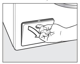
■ Open the drain pump access panel.
