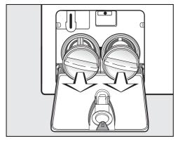
■ Remove the drain filters completely.
